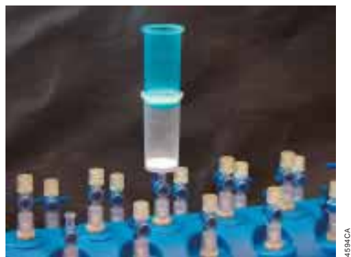
Figure 5. Proper assembly of the PureYield Clearing Column (blue) and the PureYield DNA Binding Column (white) for use with the vacuum protocol of the PureYield Plasmid Midprep System.
