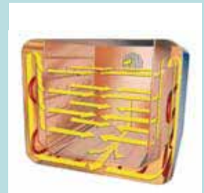
APT.Line®, air circulation mechanical convection
