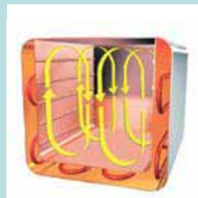
APT.Line®, air circulation natural convection
